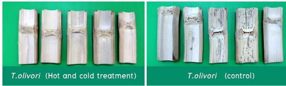
Figure 3. Damage by insect on treated bamboo and their control
